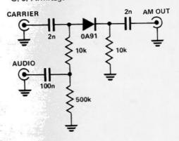
A very handy device around any hobbyists workshop or serviceman's bench is a simple modulator. For aligning IF amplifiers, receiver front ends etc — especially with only basic test instruments, it's a must.
